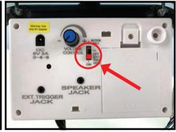
Move the switch to the ON position. Move in front of the item or make a loud sound (clap) to activate the item.
