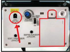
Plug in the 6V 2A ADAPTER (included) or insert 4 AA BATTERIES (not included) into the battery compartment located on the CONTROL BOX.
