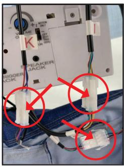
12. Attach the wires to the CONTROL BOX.
