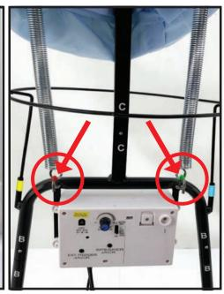
11. Attach the springs from the HEAD AND BODY to the frame on the CONTROL BOX.
